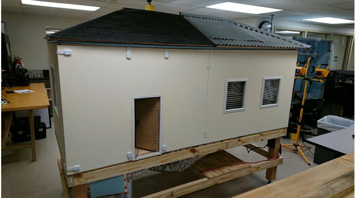
Figure 5: Highly detailed HANS system utilizing 1:4 scaled single pane glass windows, realistic stucco finish, scaled 3 tab shingles, and scaled galvanized roofing sections
