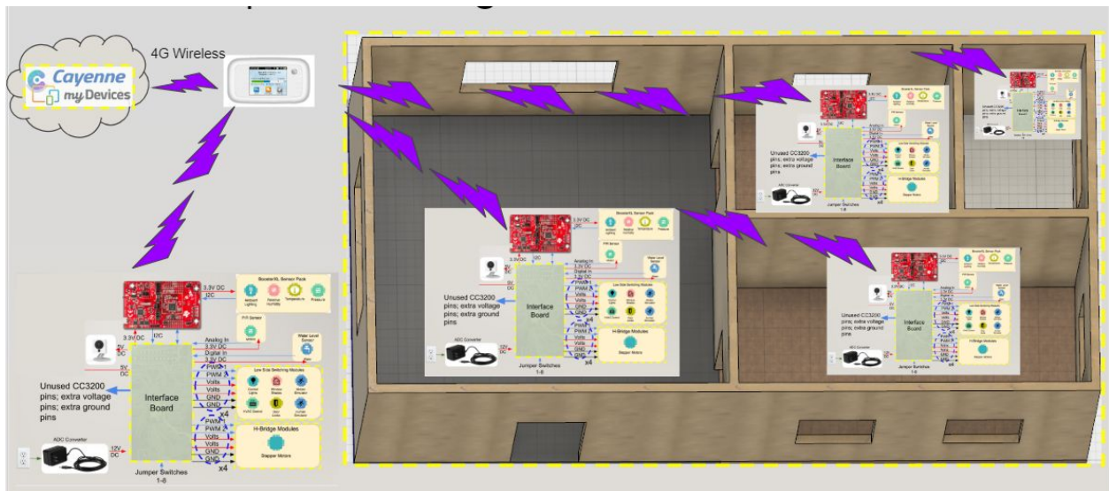
Figure 2: Conceptual block diagram for HANS showing system of systems integration across independently controlled room and environmental sensing and control modules
