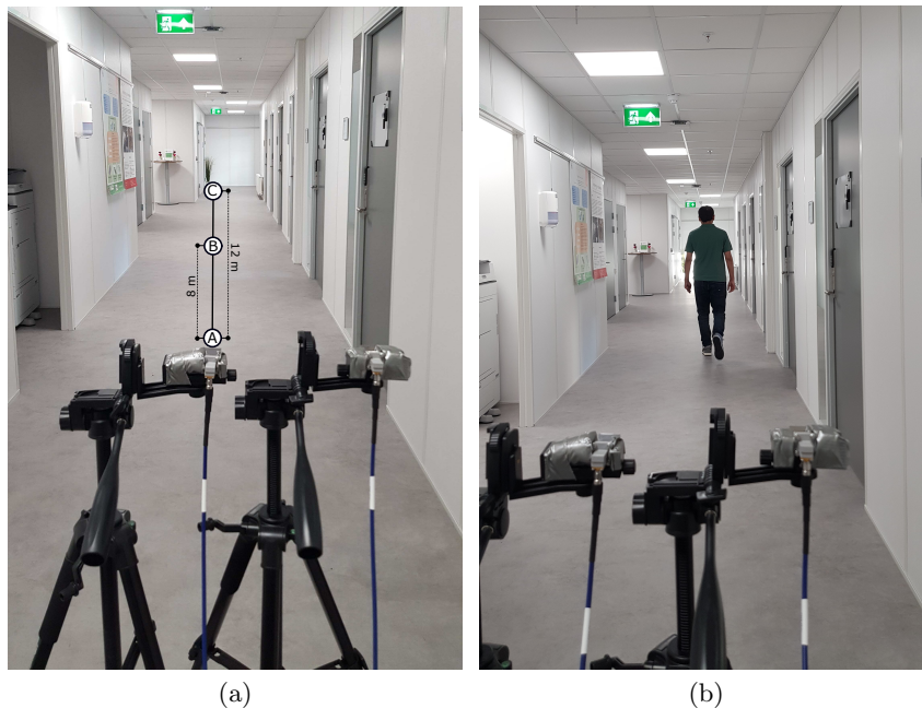
Fig. 3. Indoor radar sensing of a person walking along a floor: (a) antenna configuration and (b) walking activity.
