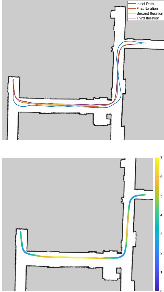
Fig. 6: Iterative approach to generate trajectory over Clemson Fluor Daniel Basement Map
