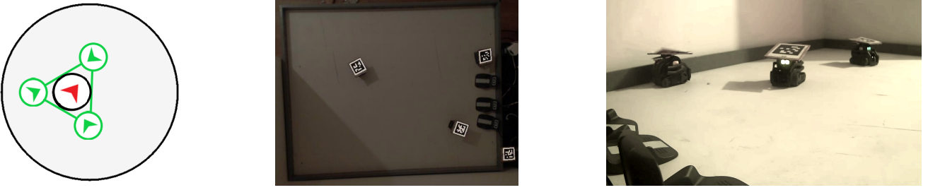
Fig. 2 (LEFT): Example of pursuer agents (green) encircling evader (red) within control circle. (MIDDLE): Real-time overhead view of Vector robots from external tracking camera, tracking robots via AprilTags. (RIGHT): Anki Vector robots in testing environment. The Vector robots are used to test our algorithm in the real-world in real-time.
