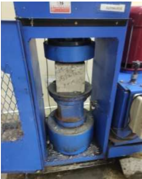
Figure 5: compressive strength test setup and cube specimen detail
