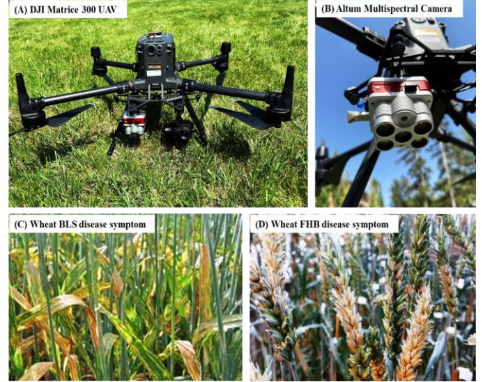
Fig. 2. The UAS platform (A) and Altum multispectral sensor (B) used in this work; photos of wheat FHB disease infected wheat canopy.
