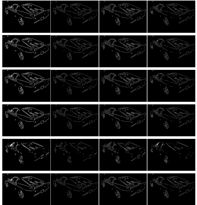
Fig. 13. Edge Filter Operator reconstructed from L1. Columns are: 3x3 kernel on L1, reconstructed using Variant 1, reconstructed using Variant 2, reconstructed using Variant 3. Rows: Sobel, Prewitt, Kirsch, Schar, Kayyali, Kroon
