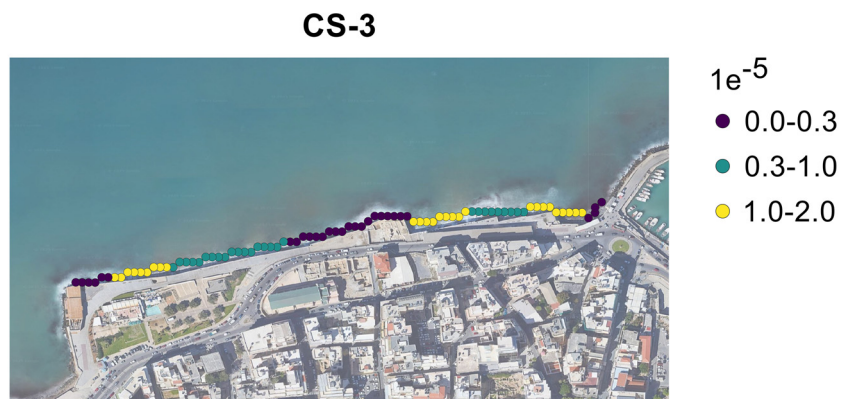
Fig. 7: Maximum value of discharges ( q , in l/s/m) computed at each point of case study 3 (Fig. 2 - Koules fortress area) (Satellite image by © Google Earth, 2023, LLC).
