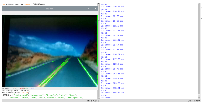
Fig 9. Canny edge detection output for straight roads and forward ultrasonic reading
