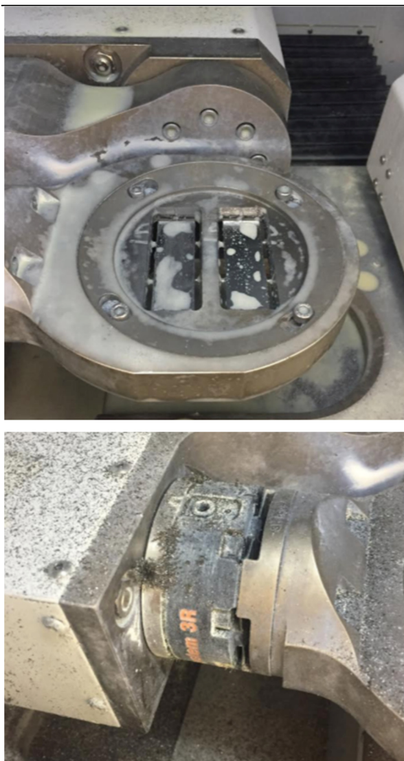
Figure 9 - 10: Steel part (or fragment ) that got magnetized during the cutting processes, and got on magnetic sensors on machine
