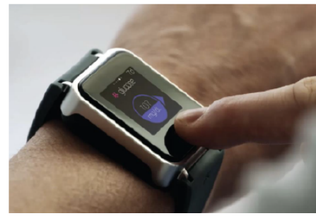
Fig. 6. Smart watch (K'Watch) to measure glucose levels [6]
