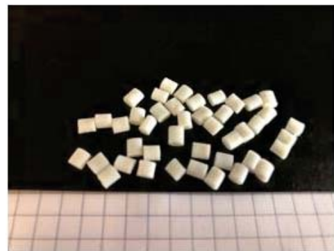
Figure 2. Photo of polymer pellets used in the capacitor sensor. Squares are 5 mm side.
