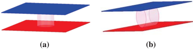
Figure 3. Parallel (a) and perpendicular (b) representations of the polymer rod between planar capacitor plates as used in 3D numerical simulations.
